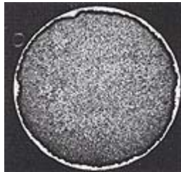
Typical cross-section, Pt Clad Mo, 0.030" * W/15% Pt, 100 x
